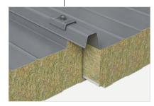
A notch in the eave area is required in order to rule out any possibility of the sheet metal shell lifting up from the insulation body (available at a surcharge). Similarly, a drip cap should be fitted in the eave area so as to prevent a capillary effect (only possible on the construction site).
